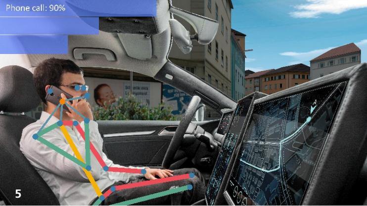
Recognizing the activities of driver and passengers for safe handovers and advanced occupant monitoring systems
